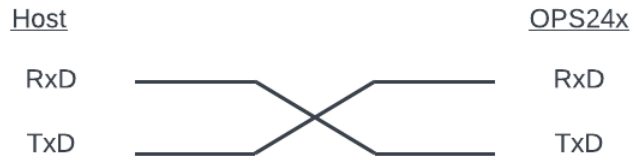
Figure 1. UART Pin Connections
