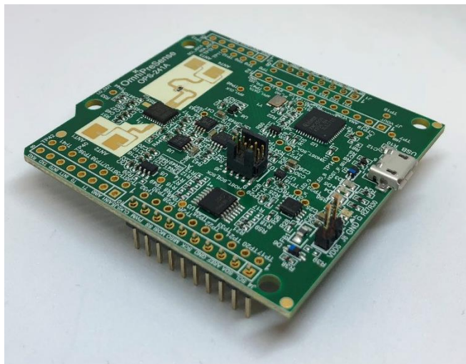
Figure 2. OPS241 with Header J1 and J4 Installed
